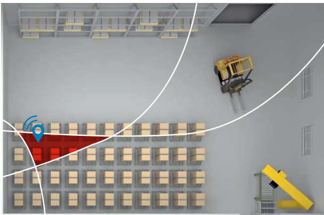
Highly dynamic RTLS: Time of Flight (ToF), accurate up to 75 cm.
